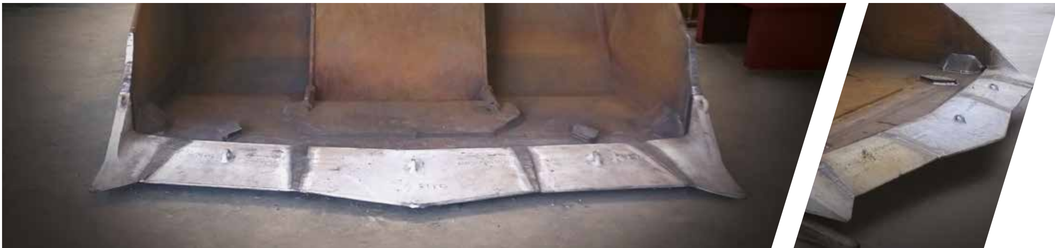
Lip for underground loaders working in Portugal.
