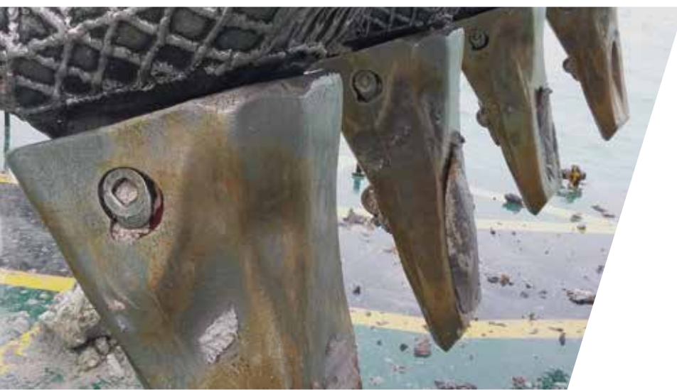
Detail of MTG Systems StarMet teeth fitted to a clamshell bucket.
