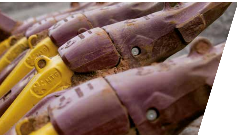
Teeth, adapters and specific shrouds for high level of abrasion and impact.
