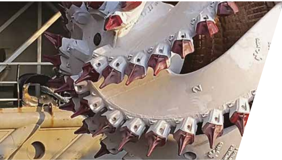
MTG Systems DMet in a MTG cutterhead working in rock terrain.
