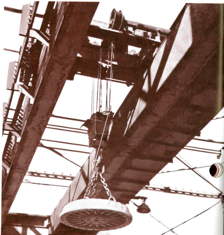
Electric cable on Rud-O-Matic® Standard Magnet Reel provides current for magnet operating from overhead crane.
