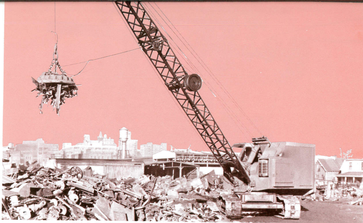
Figure A. Rud-O-Matic® Single Barrel Combination Magnet Reel and Tagline mounted on boom, operating in scrap yard.
